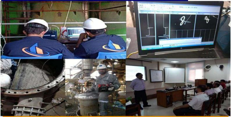
Eddy Current Testing is a fastest NDT technique among all other NDT techniques. This is used for inspection of Heat Exchangers, boilers, condensers, Fin-Fan coolers tubing's in power plant, refineries, processing plants, Fertilizers and Oil & Gas sectors. For surface inspection, it is used almost in every Industry including Nuclear, Aviation and aerospace to ensure safety and integrity of the components.
